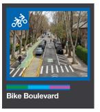
Bike boulevards are streets designed for low car and truck traffic and feature a range of safety treatments to make bicycling safer and more comfortable. These designs are still evolving, so some are
